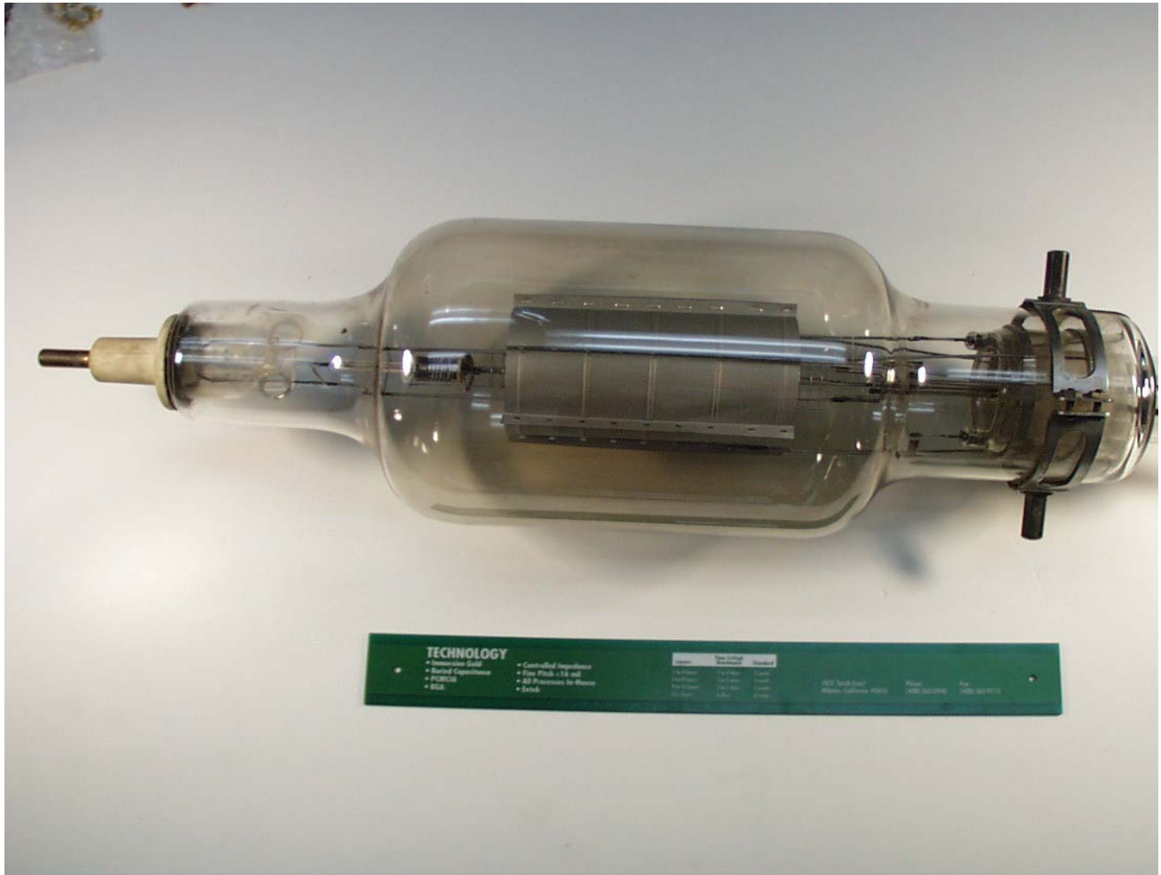
Transmitter Power tubes circa 1925, the largest glass RF power tubes still using forced air cooling system
