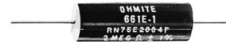
(c) Metal-film precision resistors App: Where high stability, low temperature coefficient, and low noise level desired
