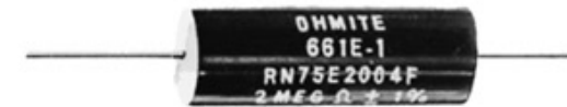
(c) Metal-film precision resistors App: Where high stability, low temperature coefficient, and low noise level desired
