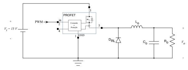
Figura 29 – Circuito do conversor cc-cc Buck.
