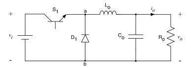
Figura 2 – Circuito do conversor cc-cc Buck.
