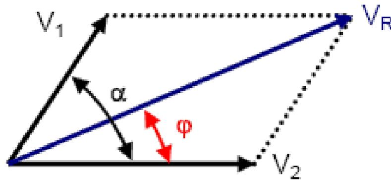
$$V_R = \sqrt{V_1^2 + V_2^2 + 2 \cdot V_1 \cdot V_2 \cdot \cos \alpha}$$
